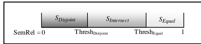
Figure 9. Basic semantic topological relationships and corresponding thresholds following [88, 89].
